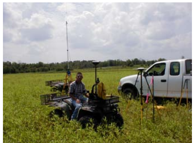
Figure 13–16 Survey-grade GPS equipment increases the efficiency of topographic surveys
